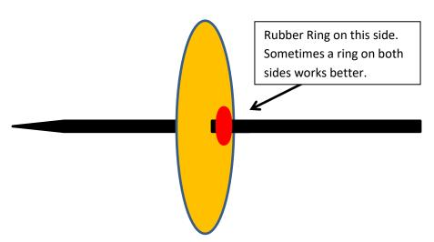
Keep a couple of made up spotters for instant use when they get a shot through them. Repair holes in the spotter immediately after they occur!! Save the repaired spotter as a spare. Two styles of pegs are supplied. Choose which works for you.
